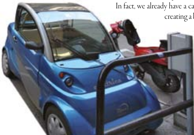
Low Speed Vehicles appropriate for Village use. Here in Italy an electric quadracycle and motorscooter charge at a municipal, on street charging station
